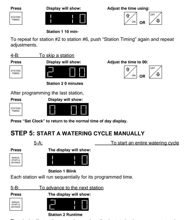
The clock will stop the manual operation after last station has run or you touch the "AUTO/OFF" button.
