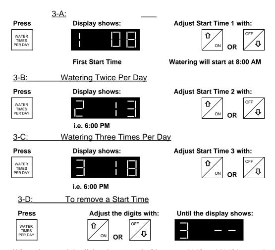
When the two right digits change to "--" between "23" and "00" hours, the start time is eliminated.
